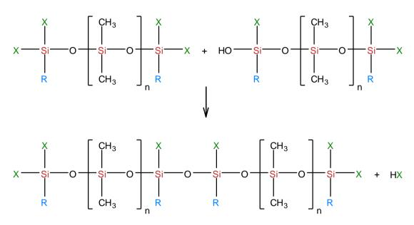
Repeated hydrolysis and reaction of resultant polymer end groups lead to full cure with elimination of HX as a by-product of the condensation reaction.
