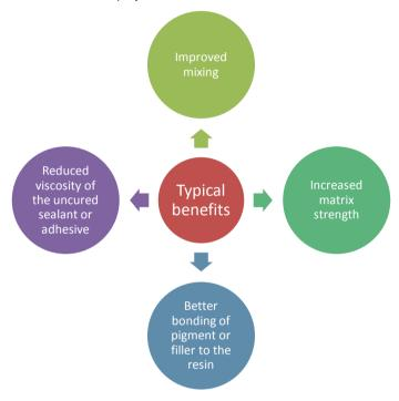
The filler may either be treated with silane before it is added to the sealant formulation (pretreatment method), or it can bind with the filler during compounding (additive method).
